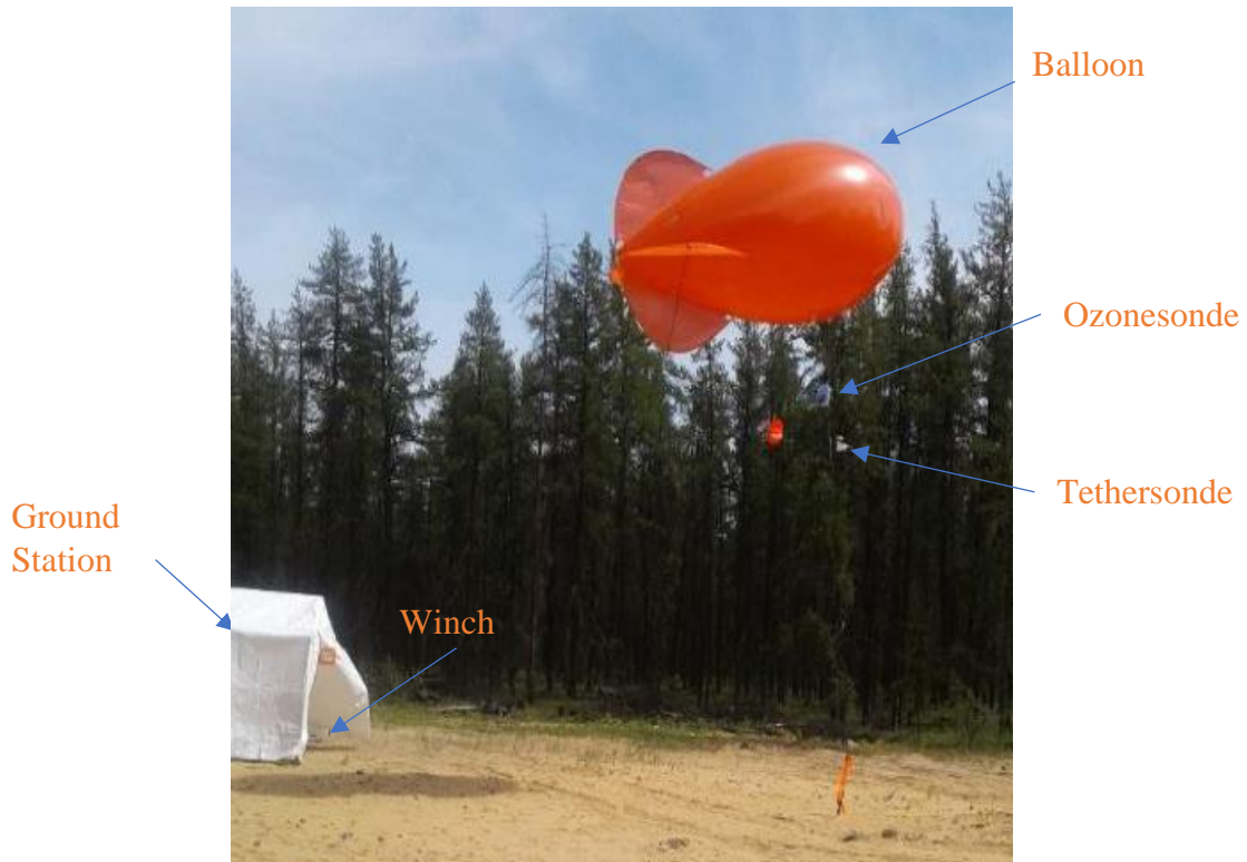
Figure 2.7 The Tethered-Balloon measurement system. This Figure includes the balloon, tether sonde and ozonesonde. The height difference between ozonesonde and tether sonde is about 15 cm. The ground station, antenna and winch are in the white shed.
