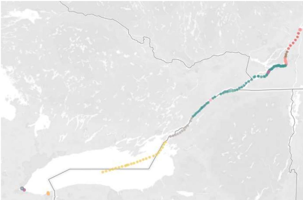
**Figure 4–38.** Final AIS Clusters resulted from the proposed clustering framework in Lake Ontario and St. Lawrence River, with each color representing one vessel behavior pattern
