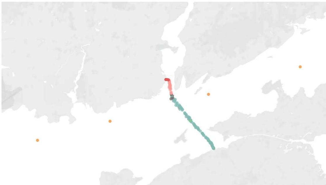
**Figure 4–37.** Final AIS Clusters resulted from the proposed clustering framework on the location between Kingston to Port at Wolfe Island, with each color representing one vessel behavior pattern
