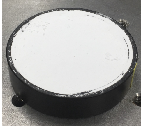
(c) Alumina 2.1 \mu m Sample
