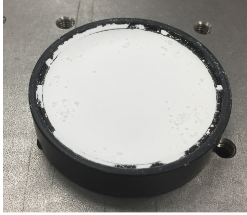
(a) Alumina 0.1 \mu m Sample
