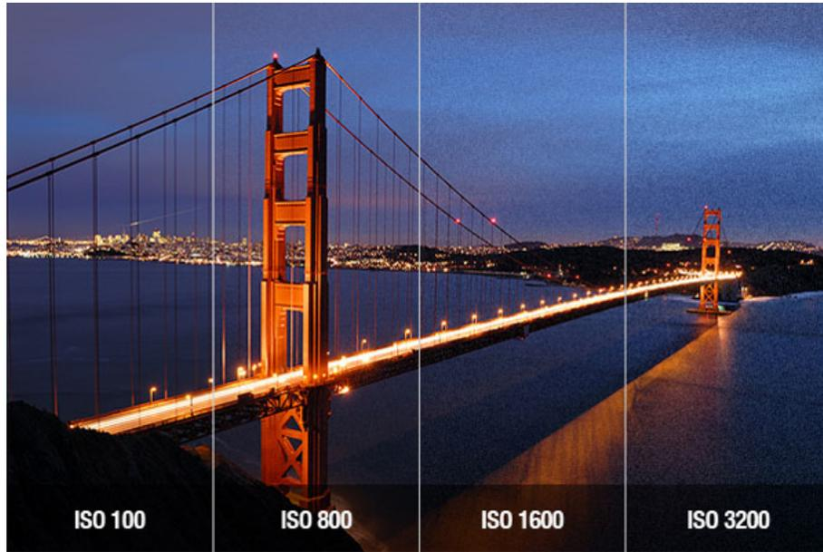
Figure 2.5: A simple illustration of sensor gain and ISO level showing an image captured under different ISO levels. It is observable that the higher the ISO, the higher the noise.
