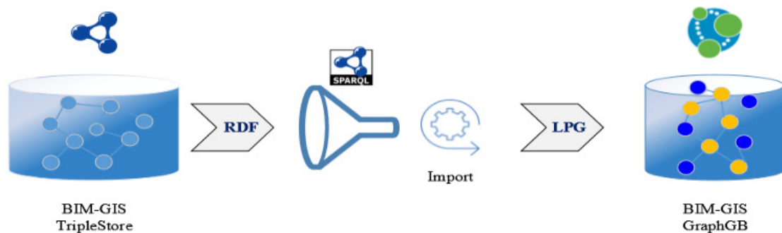
Figure 5.2 RDF transformation and loading pipeline
