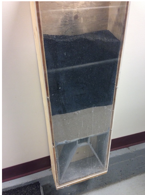
Image 1: A model of the sand filtration system used to filter Iqaluit's water (Photograph by Victoria Watson)
