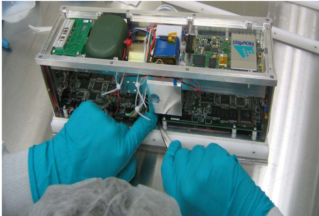
Fig. 3.2. The front-end view of Argus 1000 engineering model mounted on the CanX-2 nano-satellite [Source UTIAS].
