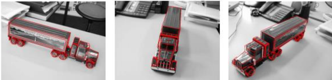
Figure 4.2. Example of edge-based tracking using a toy truck (Wuest and Stricker, 2007).
