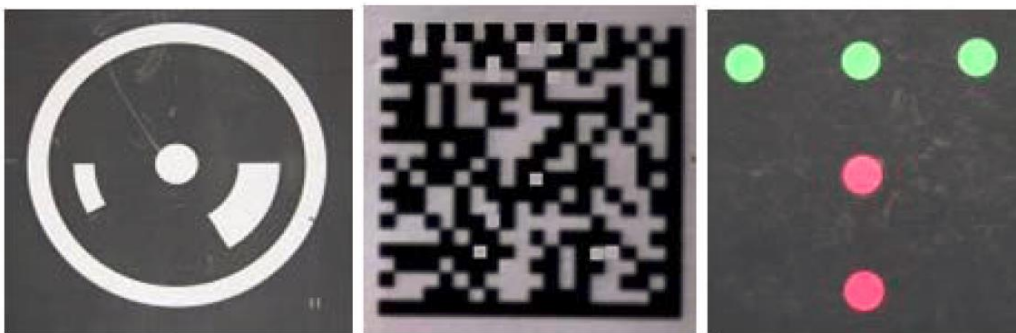
Figure 4.4. Three examples of coded targets used for point identification and camera calibration (Mautz, 2012).
