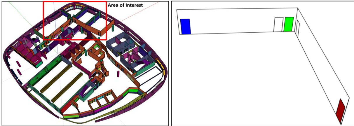
Figure 5.28. Left) The 3D indoor model of the second floor in the Bergeron Centre. The area of interest of the second experiment is outlined by the red box. Right) The 3D wireframe model used in the second experiment.
