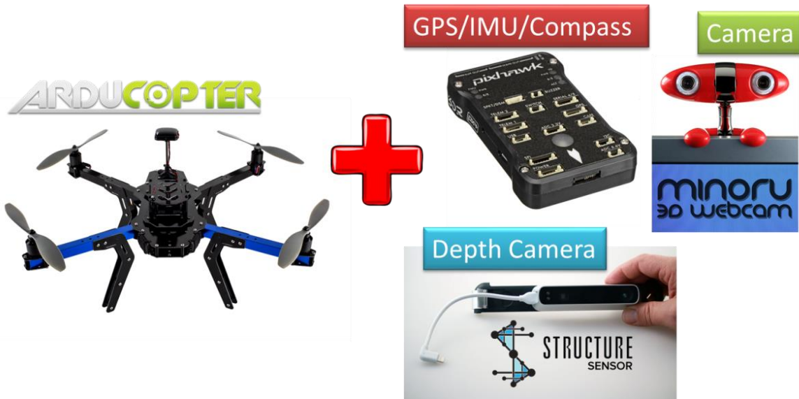
Figure 5.14. Components of the developed indoor/outdoor UAV.
