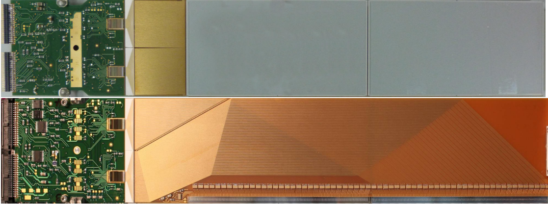
Figure 3.1: ALPHA SVD hybrid. Front view (top): the silicon sensors are connected to the ASICs (Application Specific Integrated Circuits) through bond wires, which are the path of the p-strips signals (see text). Rear view (bottom): n-strips connected to the ASICs. In both views the PCB (Printed Circuit Board) and the four VA1TA ASICs mounted on it are clearly visible. Credits: JTMK.
