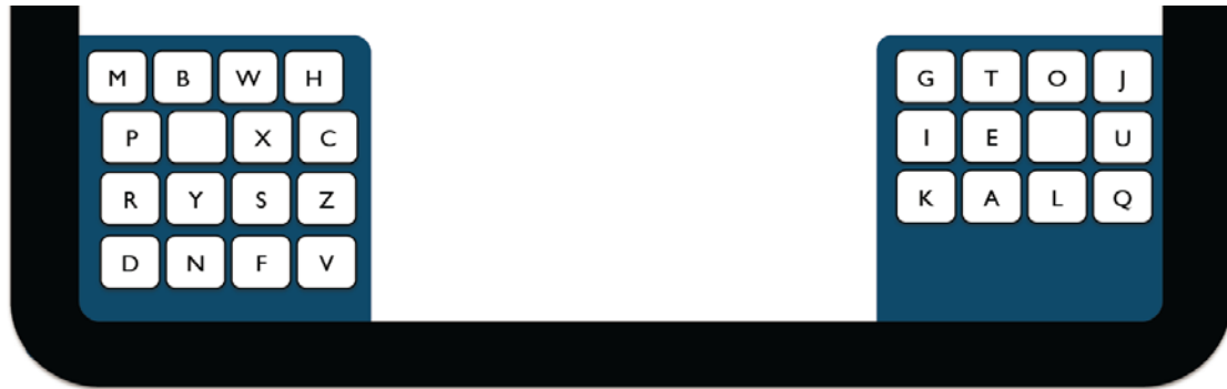
Figure 26. The KALQ keyboard [83] uses a split, modified layout.
