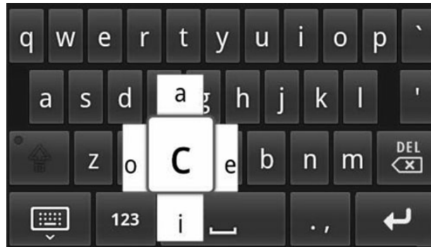
Figure 27. The KeyScratch keyboard [30] combines tapping with multi-letter gesture input on a popup menu.
