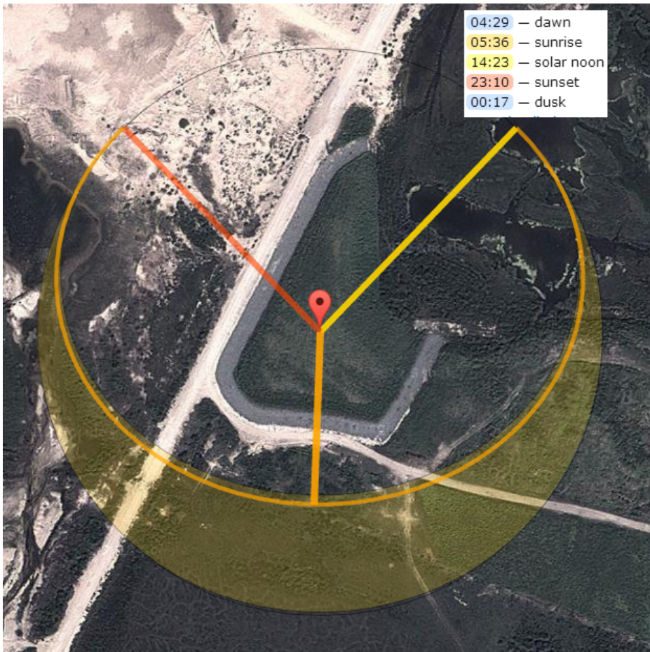
Figure 2.13.1. Mid July sun exposure at the old Churchill dump. The central feature, surrounded on three sides by light grey is the berm. Reading clockwise from the teardrop map marker the line oriented at 2 o'clock is the dawning sun horizon position. The line oriented at 6 o'clock is the solar noon position and the last line is the setting sun horizon position. The width of the pale crescent indicates the amount of sunlight received. Image retrieved from "www.suncalc.net".
