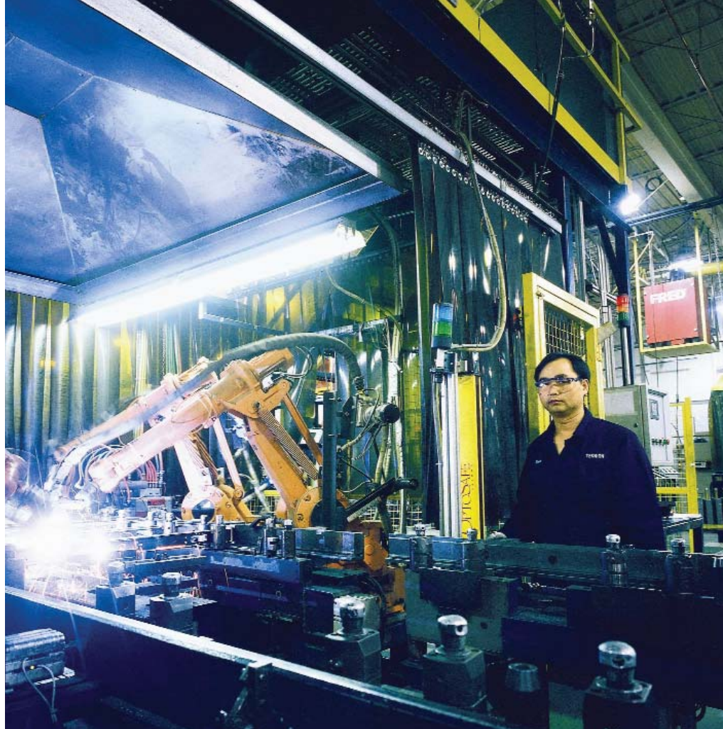
Welding has undergone extensive examination and process redesign at Teknion, through ISO 14001 certification, to ensure minimal or no impact is made on the environment. Water is recycled and used for cooling the machinery, the air is drawn out of the welding area to filters, cleaning the air enabling it to be recirculated and a materials reduction program minimizes the amount of waste created. Photo: Teknion.
