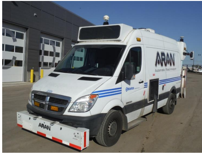
Figure 2.1 - Automatic Road Analyzer (ARAN) (City of Edmonton 2021)
