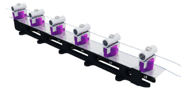
(b) SMA wire actuator mounted to steel beam external from hand
