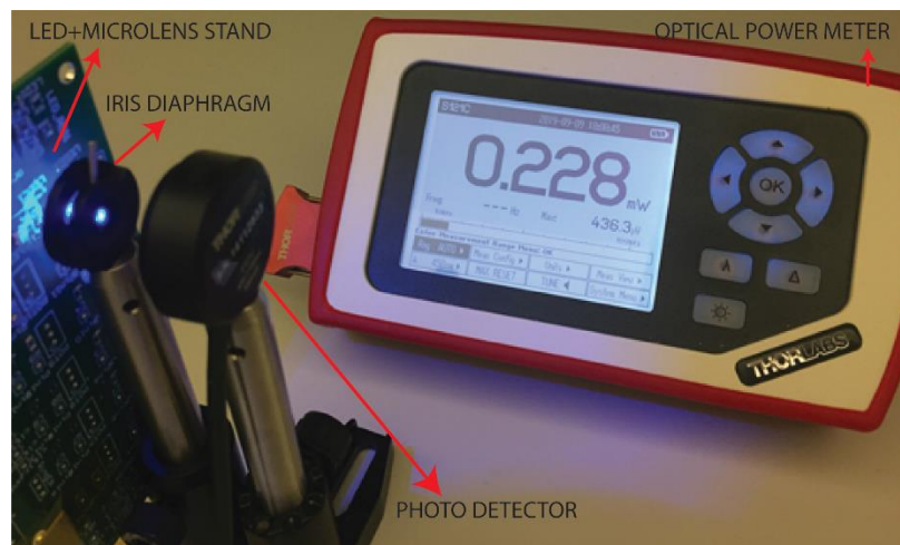
Figure 4.10: Optical measurements setup.
