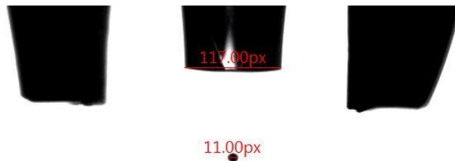
Figure 4.9: Drop diameter calculation in comparison with nozzle diameter.
