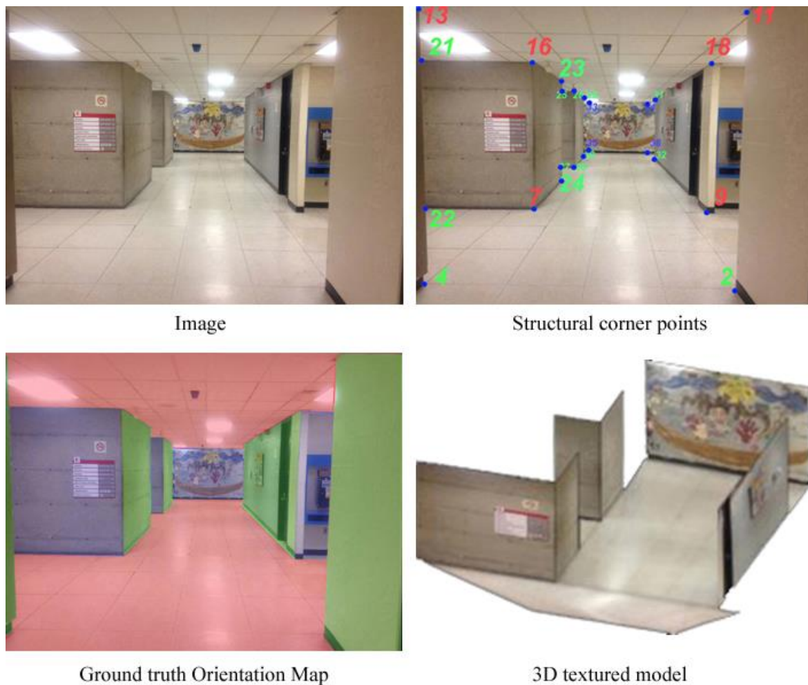
Figure 3.3 Ground truth orientation map and indoor corridor 3D model associated with a sample image from the prepared dataset.
