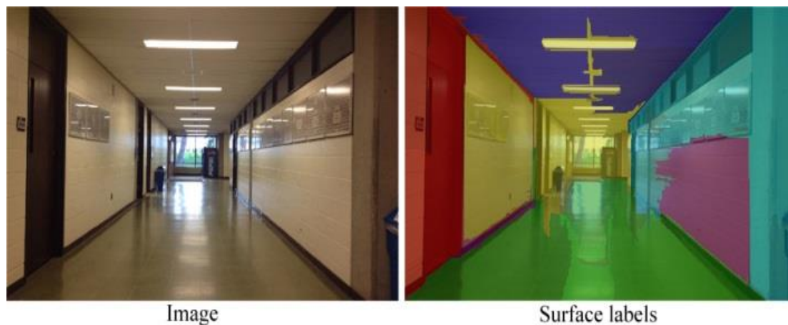
Figure 4.4 Single image of an indoor corridor and the estimated surface labels shown by different colors.
