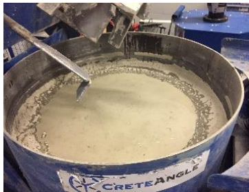
Figure 3-22 Addition of the liquid material in one phase during step 2
