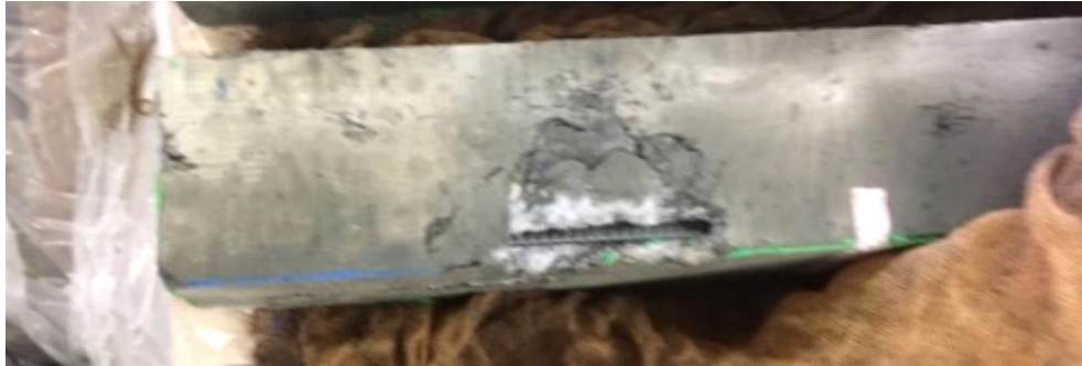
Figure 4-27 Poorly consolidated beam from batch C3
