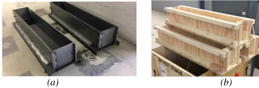
Figure 3-6 (a) Steel and (b) wood formwork
