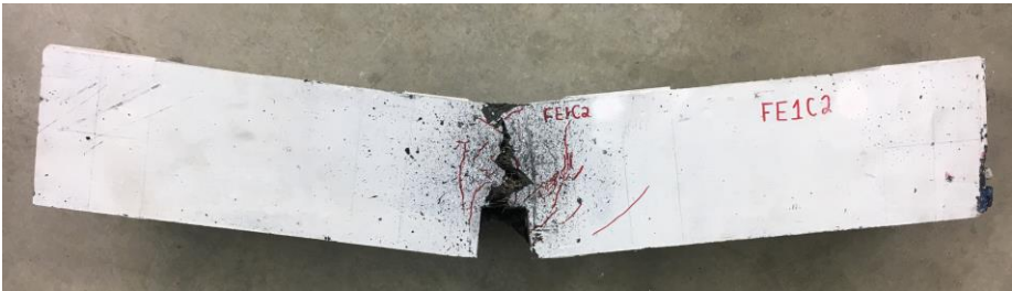
Figure 5-30 Crack pattern after failure - Beam FE1C2
