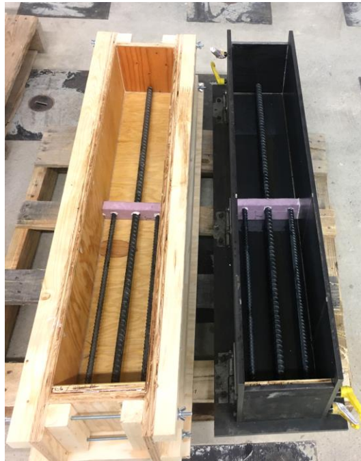
Figure 4-14 Setup for the fully bonded beams
