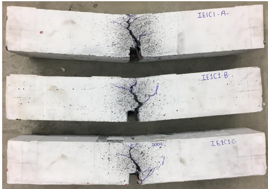
Figure 5-36 Crack pattern after failure - Beam IE1C1
