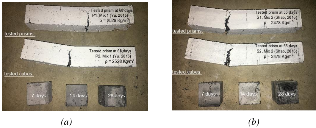
Figure 3-20 Failed prisms and cubes (a) M14 and (b) B4
