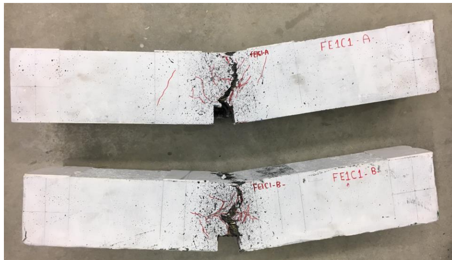
Figure 5-26 Crack pattern after failure - Beam FE1C1
