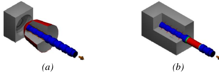
Figure 1-10 (a) Extraction of the concrete cone (b) Steel bar rupture (Ramirez, 2005)
