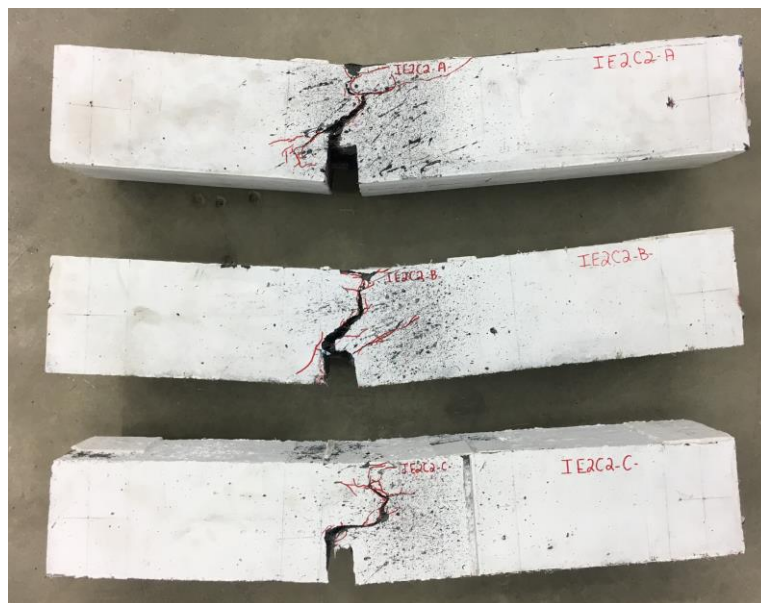
Figure 5-44 Crack pattern after failure - Beam IE2C2
