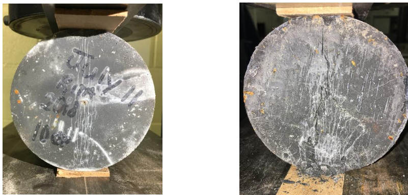
Figure 5-10 Cracking pattern for the splitting tensile test
