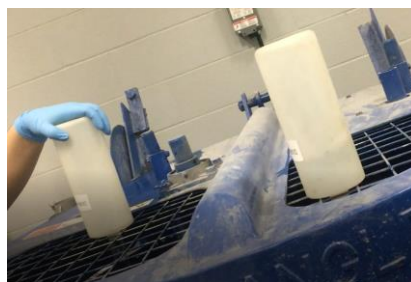
Figure 4-22 Addition of two wet mix additives to increase the flowability of the mixture
