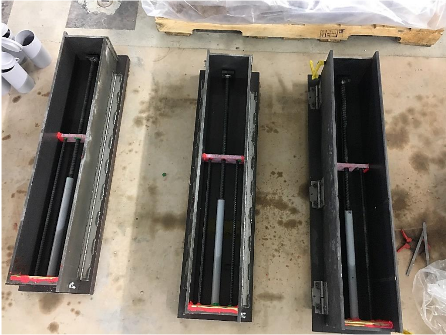
Figure 4-12 Setup for the embedment length of 10d_b
