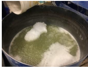
Figure 4-16 Addition of the wet additives on top of the pre-mixed dry materials
