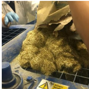
Figure 4-17 Addition of steel fibers
