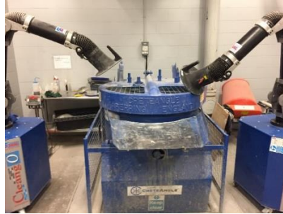
Figure 4-15 Setup of the mixing station
