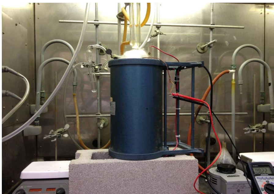
Figure 2.1. A modified reaction setup for the synthesis of hydrophobic Fe 3 O 4 nanoparticles using a thermal decomposition method.
