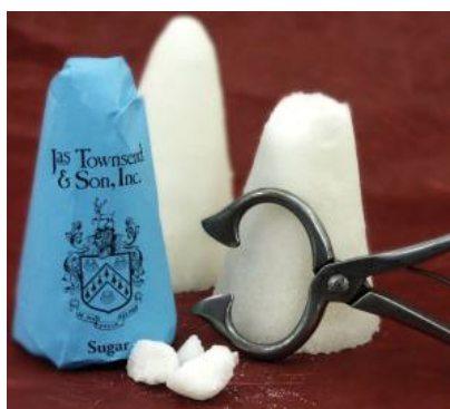
Figure 20: Sugar Nips: A tool required to cut chunks of sugar from a large sugar loaf
