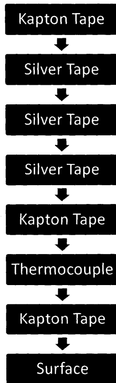
Figure 24 - Layering of Thermocouple Attachment
