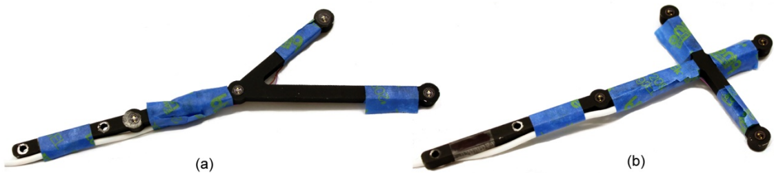
Figure 3-6: Active tools. (a) Active tool with v-shaped configuration of markers. (b) Active tool with T-shaped configuration of markers.
