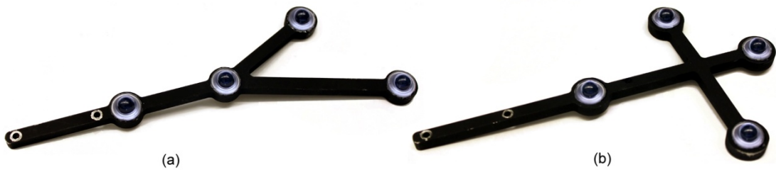
Figure 3-5: Radix tools. (a) Radix tool with v-shaped configuration of markers. (b) Radix tool with T-shaped configuration of markers.
