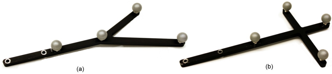
Figure 3-4: Passive tools. (a) Passive tool with V-shaped configuration of markers. (b) Passive tool with T-shaped configuration of markers.
