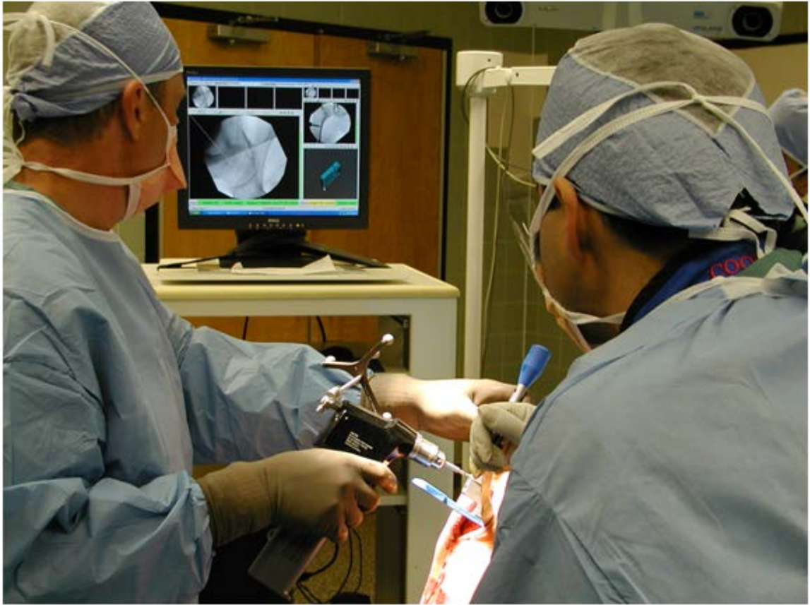
Figure 1-1: A contemporary image-guided surgical navigation system. A surgeon holds a surgical drill that is tracked by an optical tracking system (just visible in the upper right corner). The monitor displays real-time navigational information (in this case, the axis of the drill relative to the femur of the patient).
