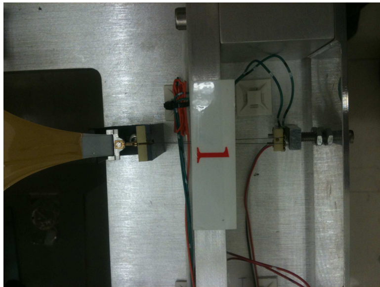
Fig. 2.4 One shape memory alloy and its attachment to the membrane and frame
