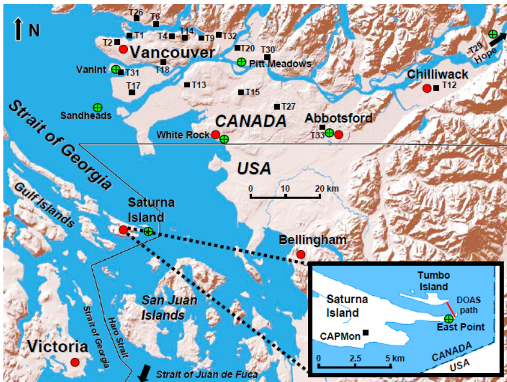
Figure 2.6: Map of the Lower Frazer Valley, showing the DOAS path between the telescope located on East Point, Saturna Island and the retro-reflector placed on the tip of Tumbo Island.
