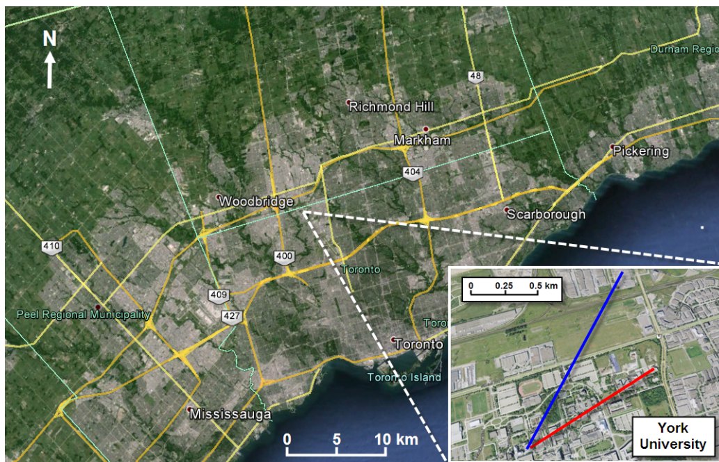
Figure 2.11: Site location for the \text{NO}_3 and HONO measurements collected at York University, Toronto. The active-DOAS light beam paths are shown in blue ( \text{NO}_3 data set) and red (HONO data set), comprising path lengths of 3.4 km and 2.2 km, respectively.
