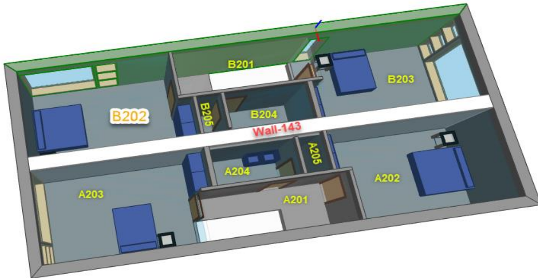
Figure 3.3. The IFC model (LOD04) includes space and wall objects
