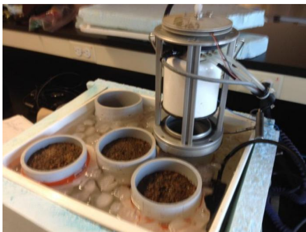
Figure 10: This set up shows the IRGA gas chamber tightly fits and sits onto the rim of which is supported 1.0 cm above the water. This image shows readings taken near 0°C with the ice bath.
