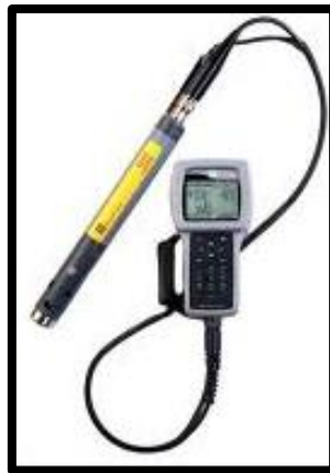
Figure 9: The YSI 600 QS probe used to instantaneously measure and record limnological characteristics of the pond water.
