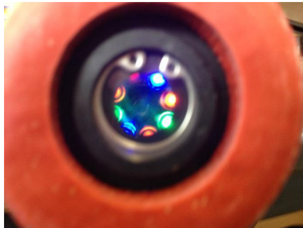
Figure 6: The different coloured LED lights that are part of the BenthosTorch detector used to excite the algae cells.
