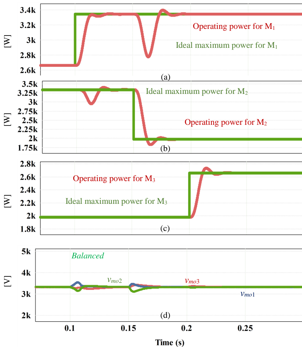
Figure 3-19 Simulation waveforms with the power balance controller: Maximum and Operating power of (a) M_1 , (b) M_2 , (c) M_3 , (d) output voltage per module.
