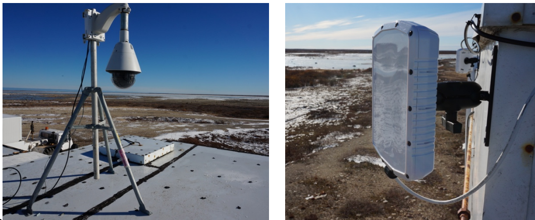
Figure 2.2. PAN-TILT-ZOOM CAMERA & RADAR PANEL. The pan-tilt-zoom camera (left) located in the centre of the radar panels. One of four C-40 D radar panels (right).
