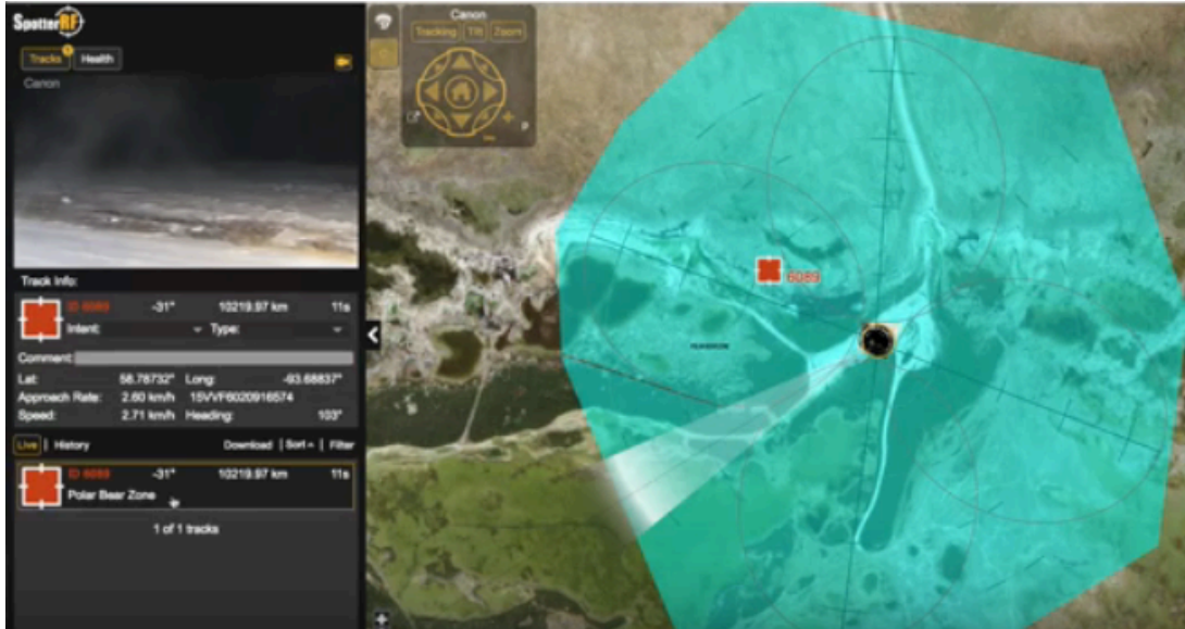
Figure 2.3. SCREEN CAPTURE OF THE ONLINE INTERFACE FOR SPOTTER RF. The online user interface shows the position of the radars, their individual ranges, and an adjustable real-time or historical log showing both geolocation of tracked objects and the camera recording.
