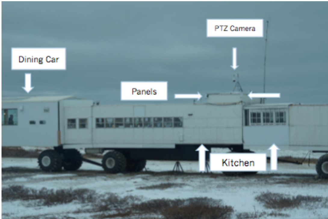
Figure 2.4. PLACEMENT OF RADAR SYSTEM. Frontier North’s Tundra Buggy Lodge shown here with the CSR system installed. One C-40 D panel was installed on each corner of the raised platform, with the PTZ camera installed in the centre of the panels, on the top of the platform.
