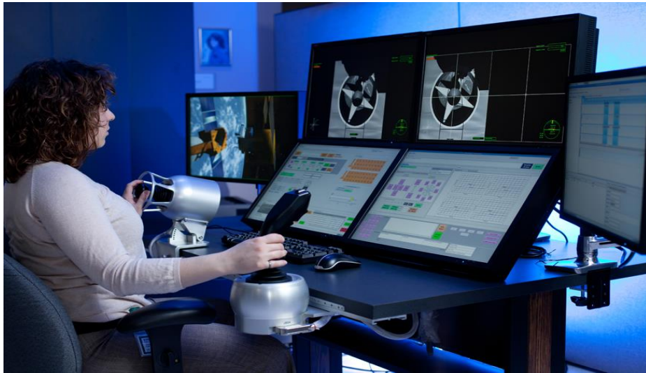
Figure 3: An operator using a joystick to control the Canadarm from the Missions Operations Station of the Canadian Space Agency. 7
