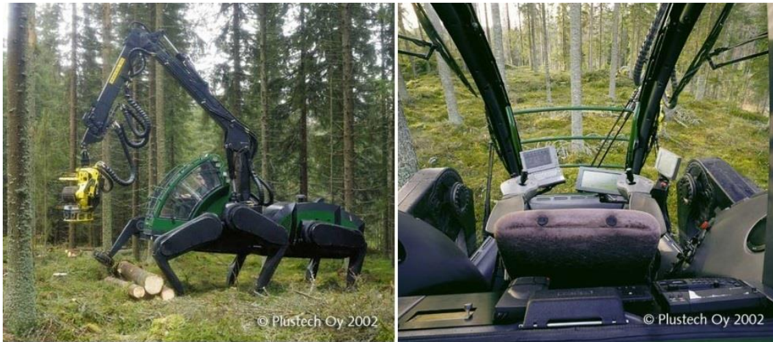
Figure 4: Plus Tech OY Forestry Excavator (left), Controls (right). 8
