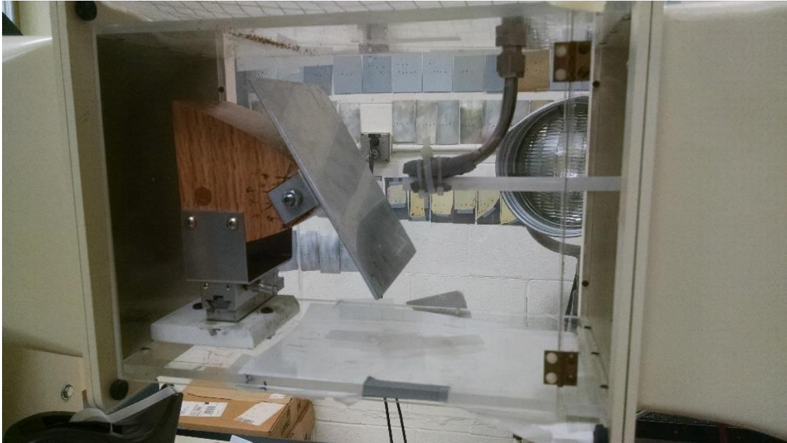
Figure 1-13 Tilted flat plate used in a wind tunnel (from Ref. [49], reprinted by permission of the American Institute of Aeronautics and Astronautics, Inc.)
