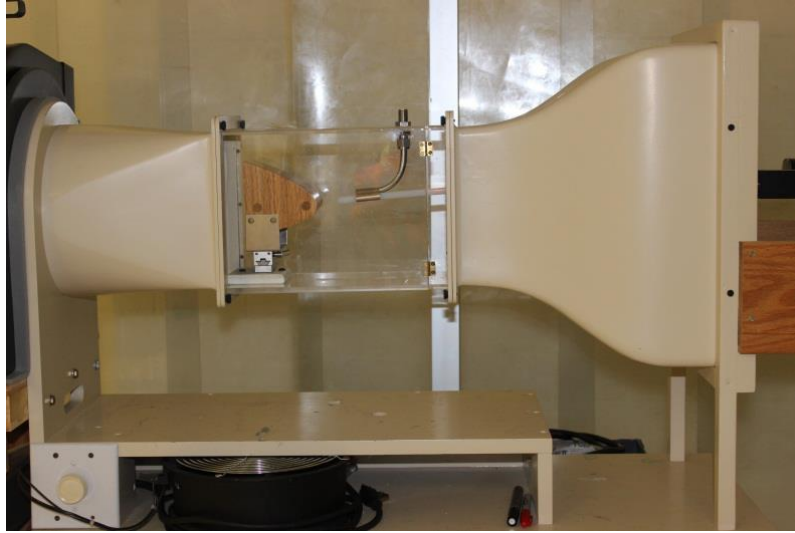
Figure 1-11 Lab-scale wind tunnel with a custom-built pneumatic gun (from Ref. [36], publicly permitted to be used by NASA)
