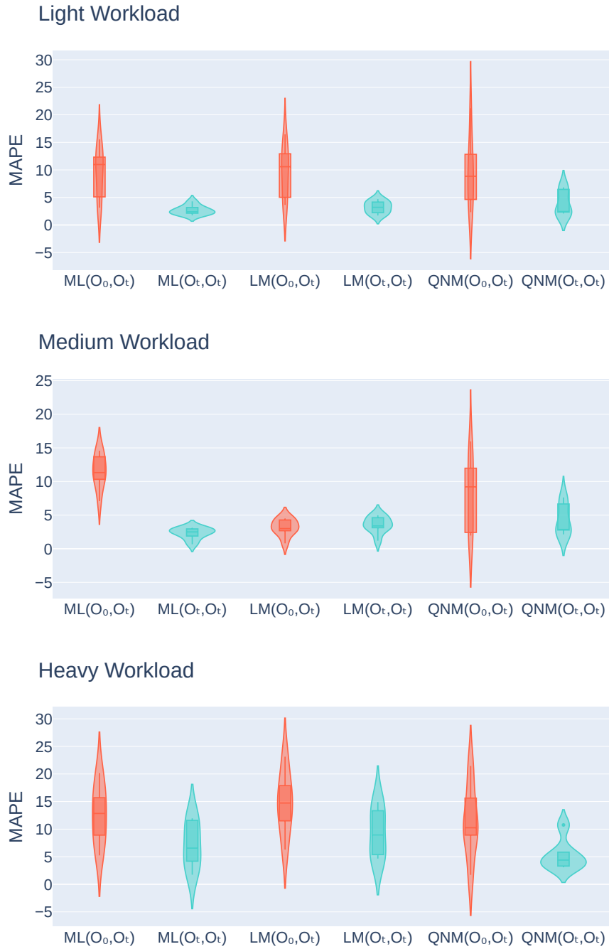
Figure 21: Prediction of Error Improvement of Co-locating Applications on 2VM Deployment
