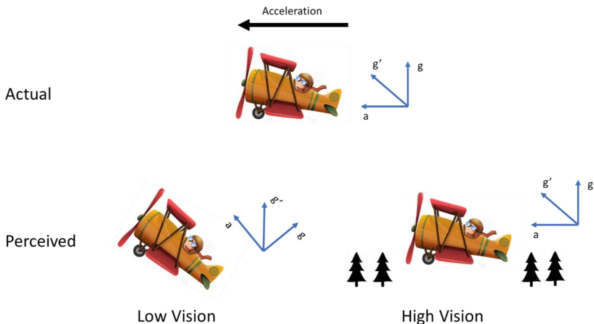
*Figure 1. 1* A diagram depicting the somatogravic illusion. The top row is the actual experience of the pilot who is accelerating forwards in their airplane. The second row shows the perceived tilt of the pilot in either a low vision condition, such as not being able to see the horizon or the ground below them, and a high vision condition where they have access to these visual cues.
