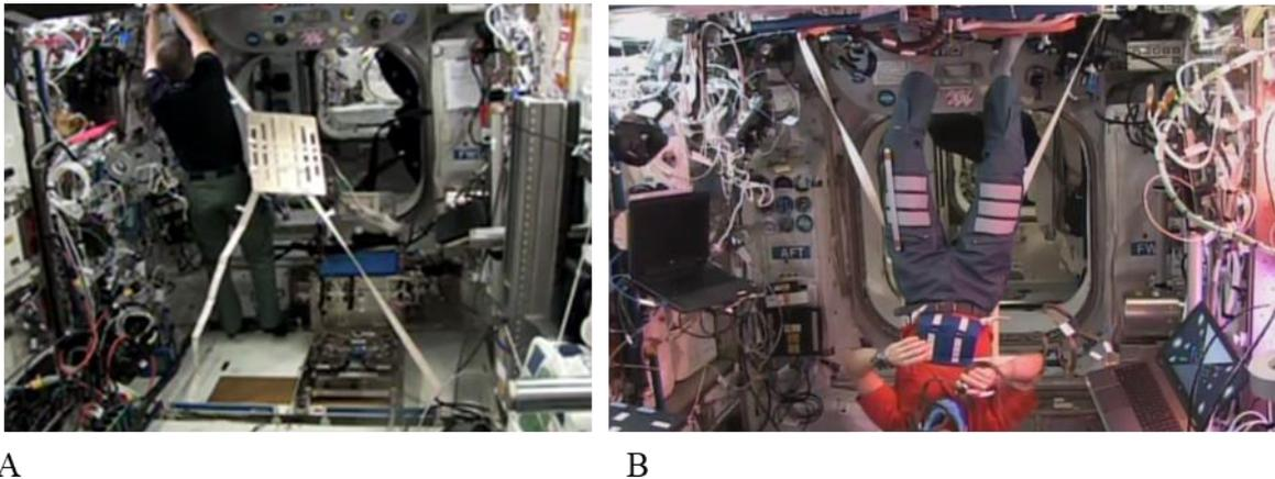
*Figure 4.2* This figure depicts the backplate. Figure 4.2A shows the backplate being set up. Figure 4.2B shows an astronaut secured to the backplate. Their head is positioned out of the picture in order to help maintain anonymity, during testing their head and feet are visible to the researchers to check that no movement or contact with surfaces takes place.
