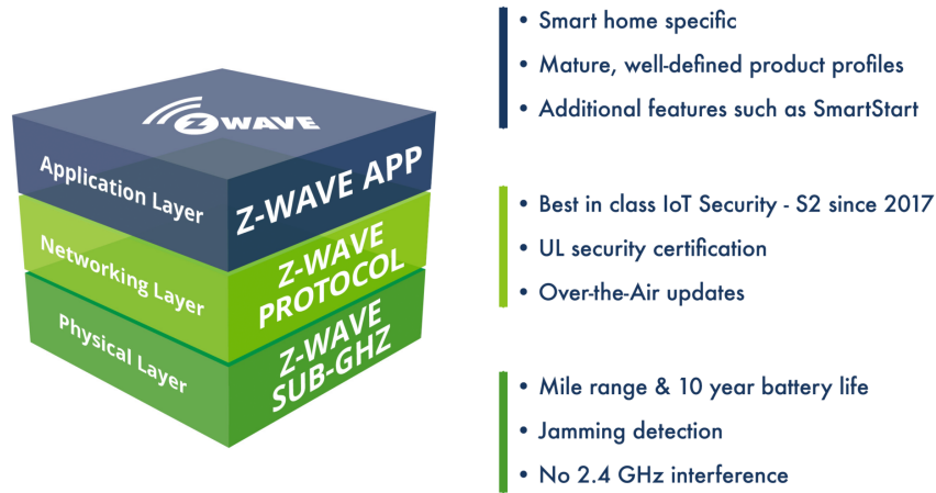
Figure 1: Z-wave protocol stack [1]
