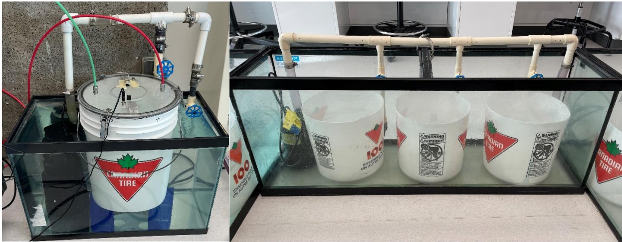
Figure 2.1. Mouse Swimming Apparatus. CD1 mice swam against a 15 L/min current generated by a submersible pump. The water current prevented floating behaviors and mice swam in pairs to minimize dunking that occurs when three or more exercise together. Pairs either swam in a closed apparatus connected to the calorimetry system (Oxymax, Columbus Instruments, Columbus, OH, U.S.A) ( left image ) or in the ‘open air’ containers ( right image ). Upon session completion, mice dried under a heating lamp.
