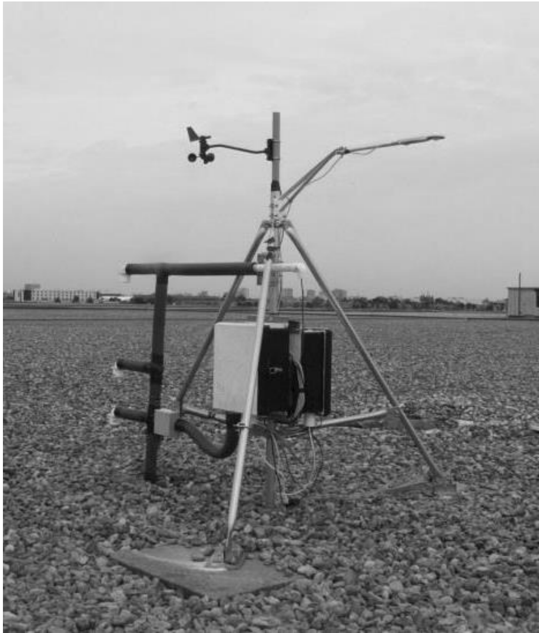
Figure 3.2. This image displays the Bowen Ratio Energy Balance system, deployed on top of rooftop at Downsview Park research site, used to calculate actual evapotranspiration.
