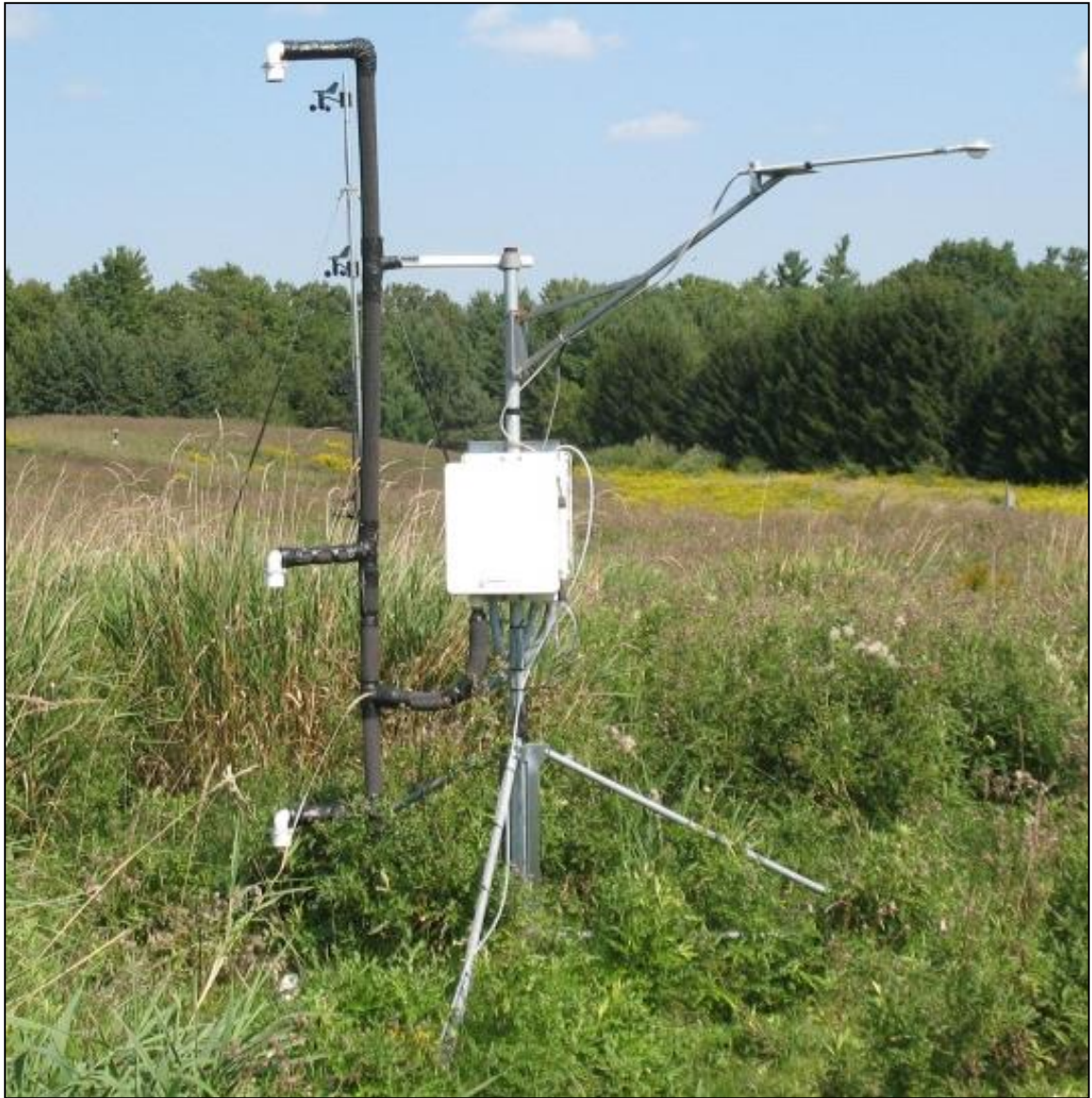
Figure 2.7. This image displays the Bowen Ratio Energy Balance system, deployed at the Kortright Centre for Conservation experimental research site used to calculate actual evapotranspiration. In the background the multilevel wind profile system can be seen.
