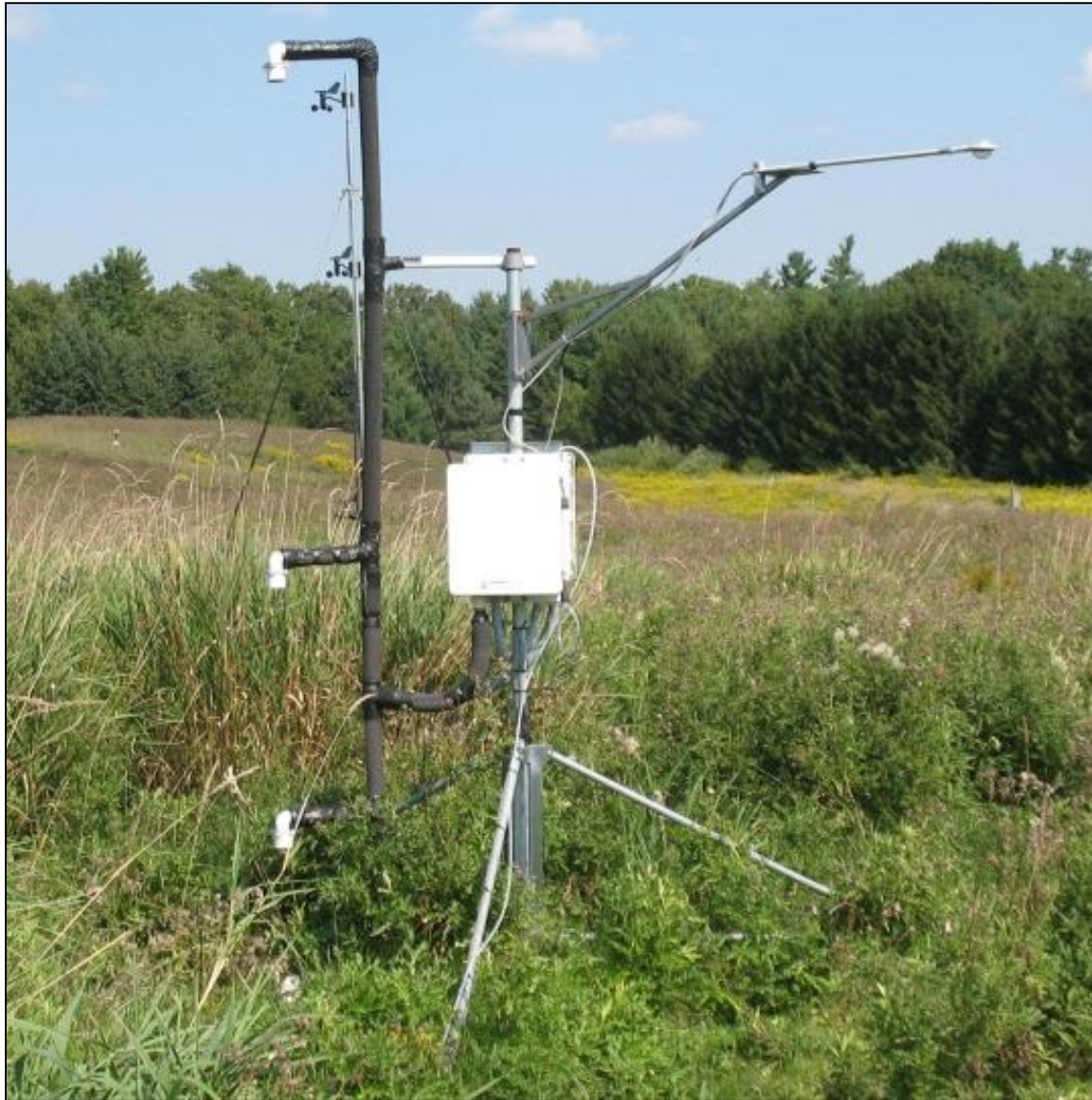
Figure 4.2. This June 2010 image displays the Bowen ratio energy balance system, deployed at the Kortright Centre for Conservation experimental research site used to calculate actual evapotranspiration. In the background the multilevel wind profile system can be seen.
