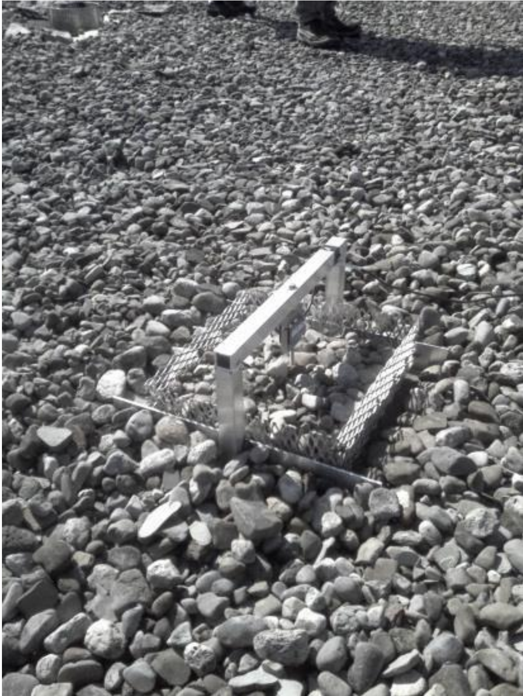
Figure 3.3. This image displays the weighing lysimeter, deployed on top of the rooftop at the Downsview Park research site adjacent to the Bowen ratio energy balance system, used to model drainage and evaporation from the roofing material.
