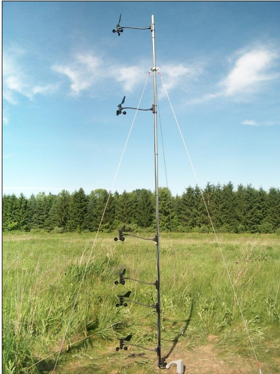
Figure 2.6. This image displays the six level, anemometer mast with Davis anemometers and wind vanes, which were used to construct wind profiles of the experimental field site. Three stainless steel guy wires are anchored to the ground and attached to the mast to prevent mast sway from wind gusts. The mast was grounded with a copper grounding wire to divert lighting strikes into the ground and away from the electrical systems.
