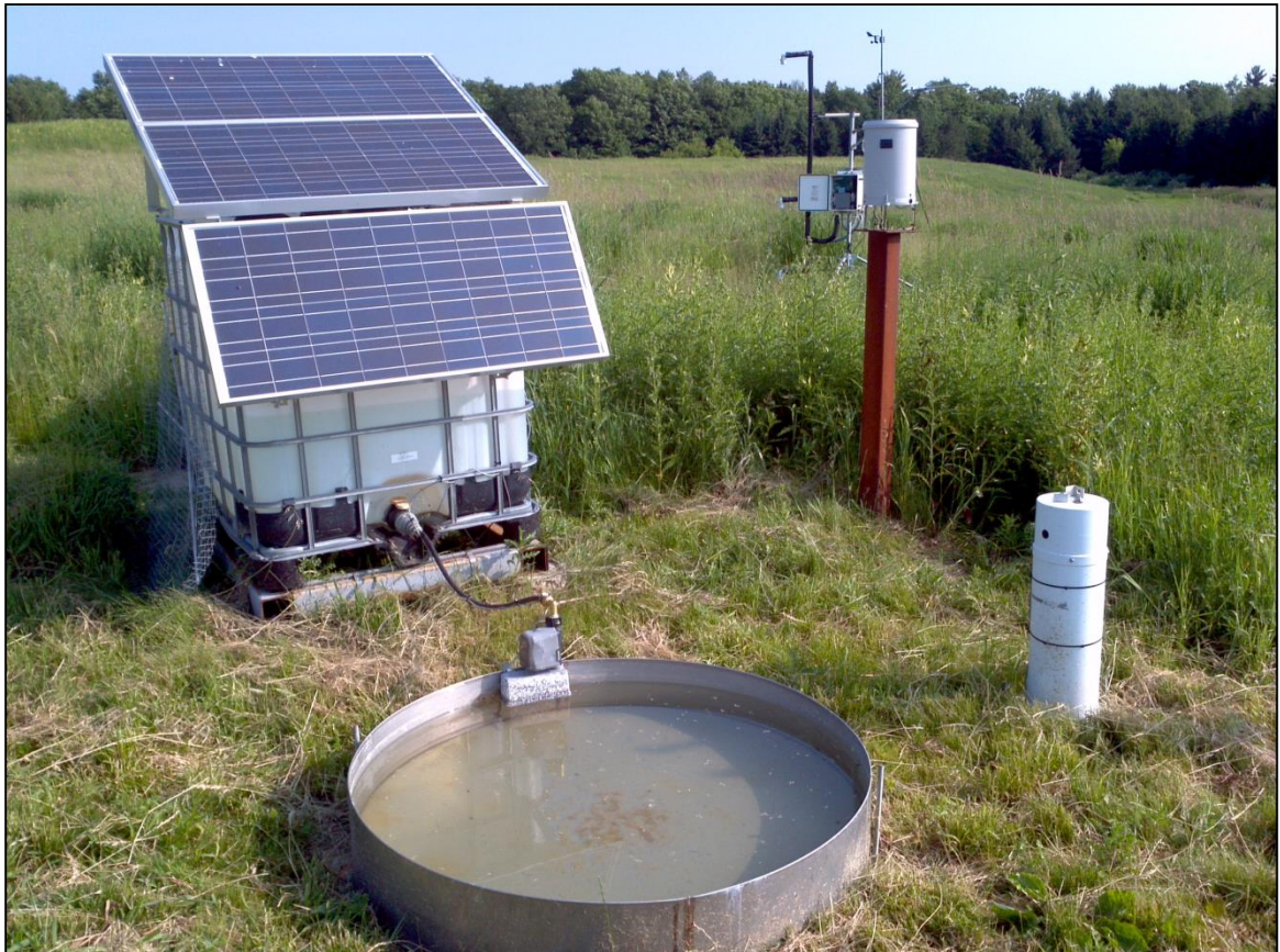
Figure 2.2. In the foreground, the Class A evaporation pan with the stilling well, water reservoir, float valve and timer, solar panels and tipping bucket rain gauge can be seen. In the mid-ground, the Bowen Ratio Energy Balance system and top of the 6 tier wind profile system can be seen.
