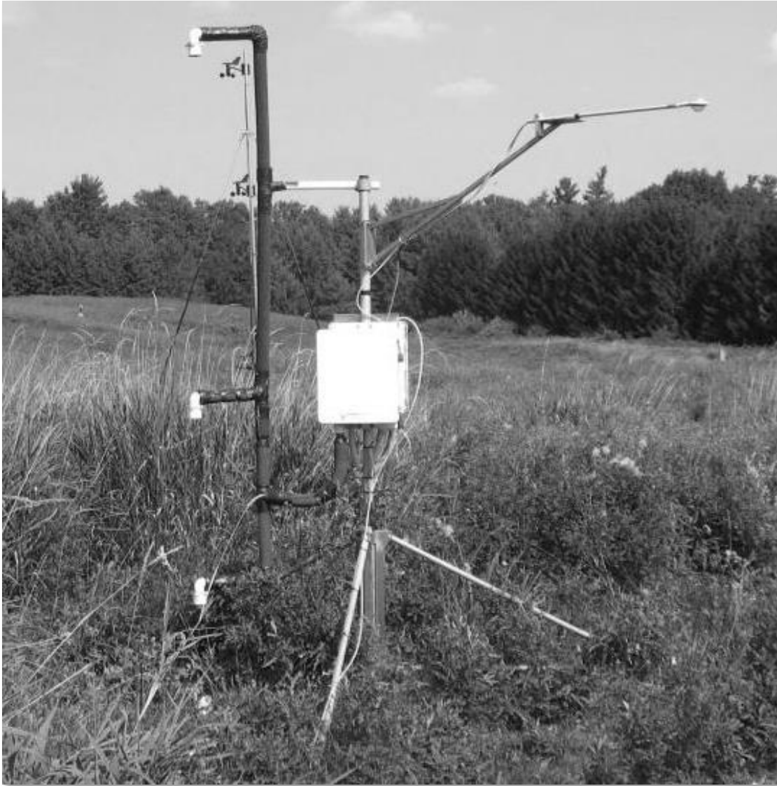
Figure 3.1. This image displays the Bowen Ratio Energy Budget system, deployed at the Kortright Centre for Conservation experimental research site used to calculate actual evapotranspiration.
