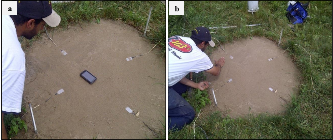
Figure 2.4. (a) displays the cardinal direction calibration of the spatial arrangement of the four Middleton soil heat flux plates used to measure ground heat flux of the Class A evaporation pan. (b) is an image of grading the mortar sand to finalize the level of the sand so the Class A evaporation pan may be positioned level with the ground and directly in contact with the soil heat flux plates.
