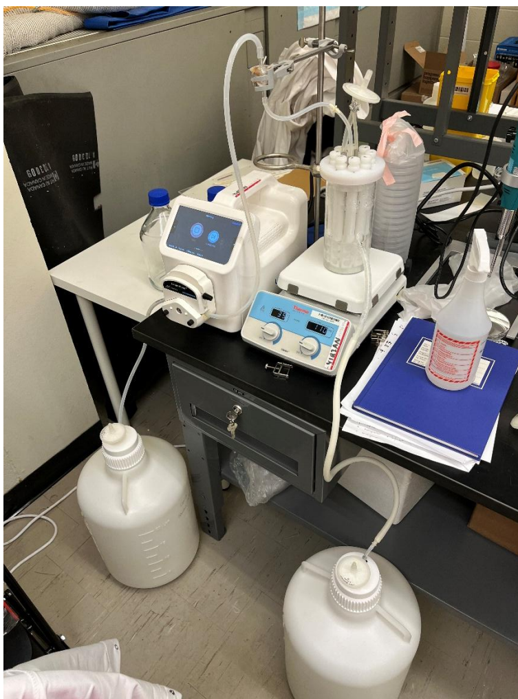
Figure 9: Fully assembled biofilm growth apparatus. Nutrient media is pumped out of the influent carboy (bottom left) and into the reactor. The CBR is attached via tubing to the effluent carboy, where excess liquid is stored once it is carried out of the reactor
