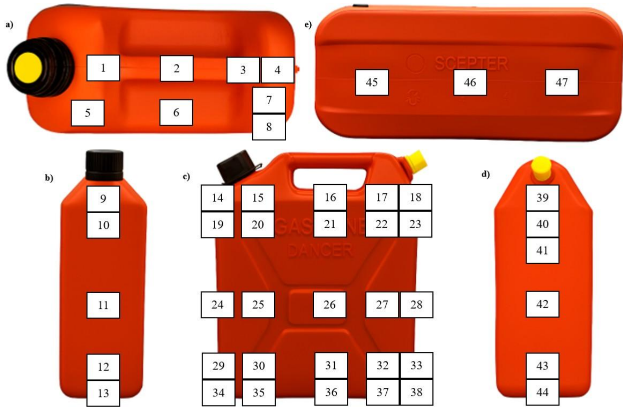
Figure 7: Hole locations in the jerry can experimental setup. Readings were taken from the a) top; b) front; c) side; d) back; e) bottom (location 34 is at the front of the jerry can while location 38 is at the back).
