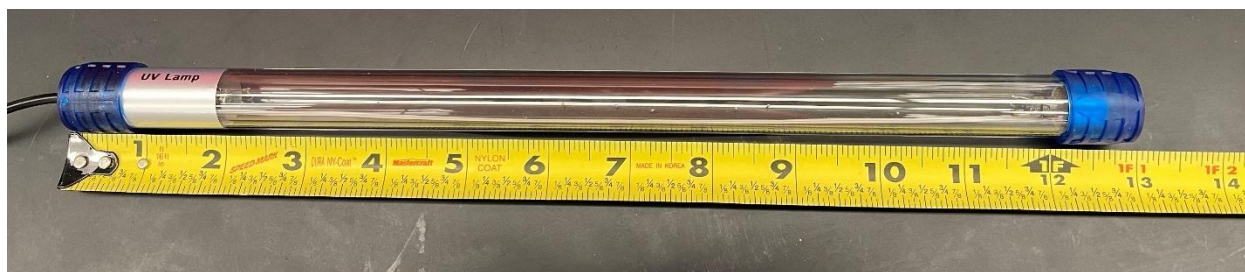
Figure 6: The UVC LED light source. UV light only irradiated from the transparent cylindrical tube.
