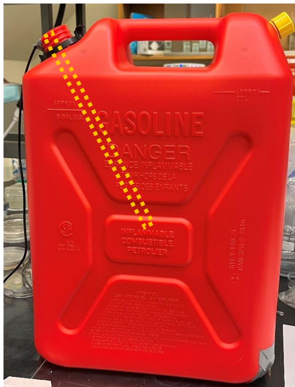
Figure 8: The yellow outline highlights the position of the UVC LED light source inside the jerry can. It was positioned at the same angle as the neck and extended to the center of the container.
