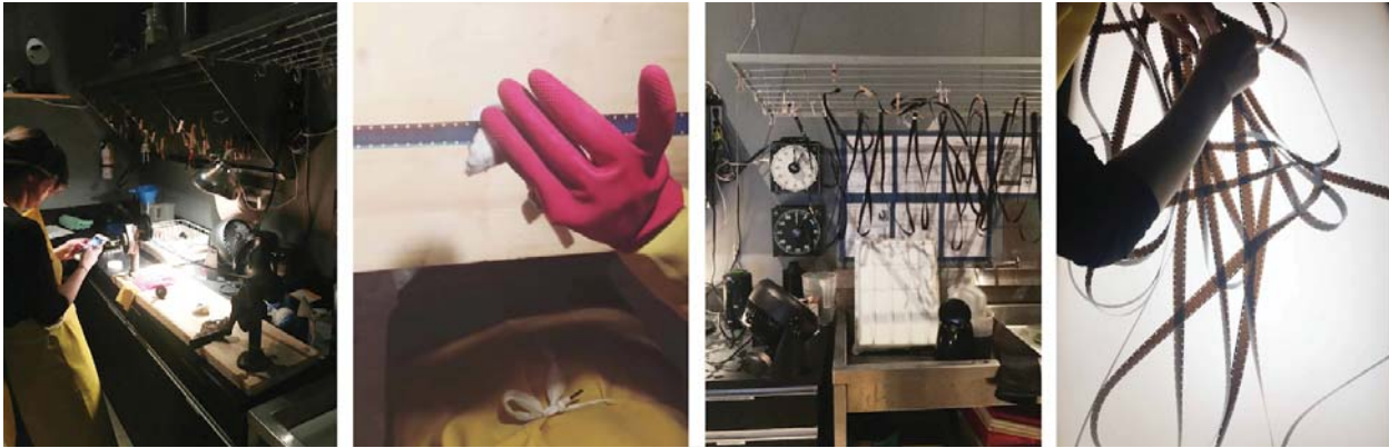
Images 25, 26, 27 and 28. Photos from left to right: Preparing to remove remjet from 16mm film, removing remjet from 16mm film with a cotton swab, leaving the film to dry on racks at LIFT and examining the results of processed film on a lightbed at LIFT. Photo credit: Rachael Watson
