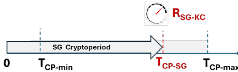
Figure 22: Impact of key-compromise Risk on T_{CP-SG} in relation to T_{CP-min} and T_{CP-max}
