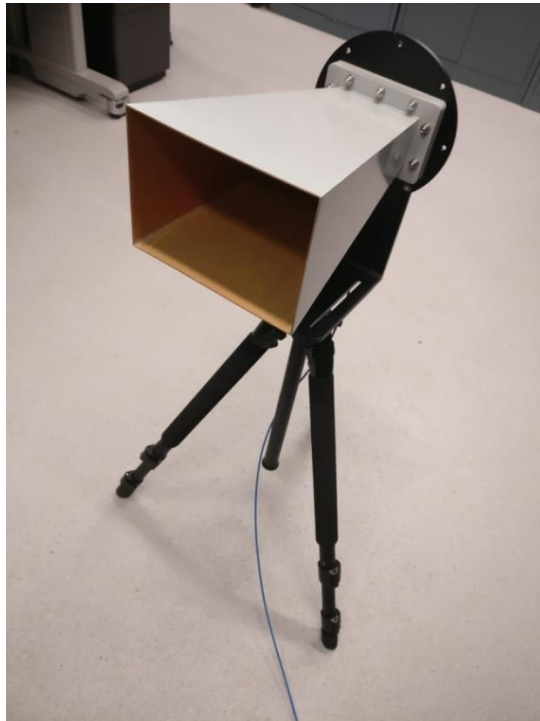
Figure 5.1: A-info P/N:LB-430-10-C-SF gain horn antenna (A-info, 2017)
