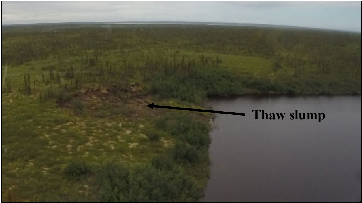
Figure 4.1: Photo of a shoreline retrogressive thaw slump on a small lake located in the uplands east of the Mackenzie Delta, and north of the town Inuvik, Northwest Territories. Photo taken in July 2017.
