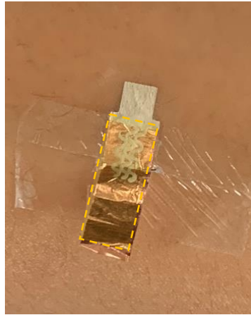
Figure 3-3. Extrusion printed square electrode with contact (highlighted) on human participant
