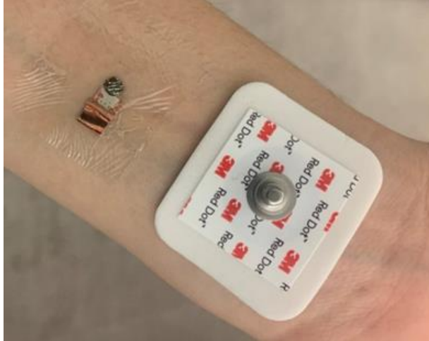
Figure 4-3. Extrusion printed circle electrode with contact and conventional electrode on left arm
