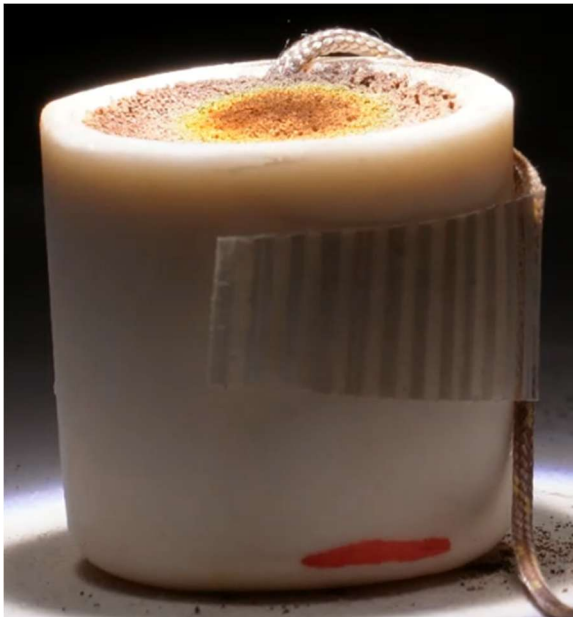
Figure 6.5: Early stage of thermal exposure showing localized discoloration.
