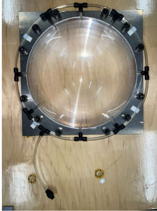
Figure 3.2: Cooling rig for Fresnel lens
