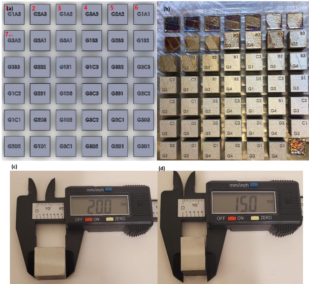
Figure 3-2. Direct metal laser sintering a) schematic of coupons before printing, b) samples after DMLS printing, c-d) sample dimension after printing
