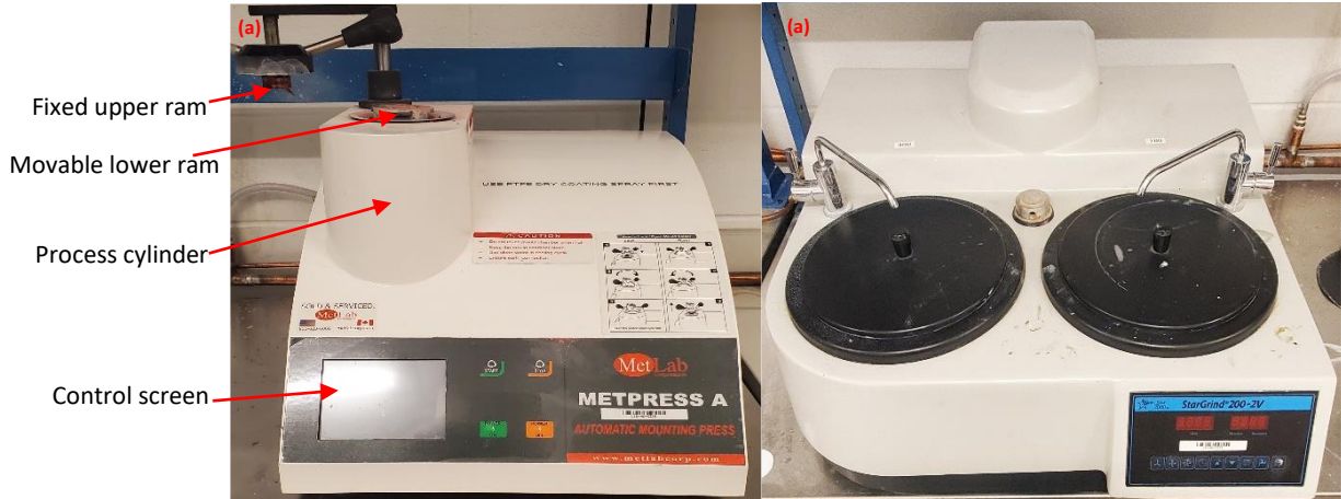
Figure 3-3. a) Hot-mounting press b) grinding and polishing station
