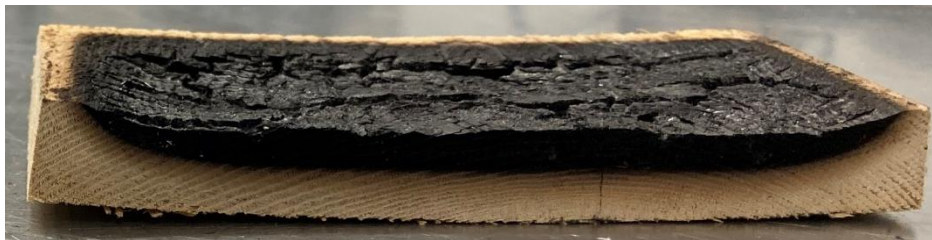
Figure 2.2: Charring on an Eastern white cedar sample (author's photo)
