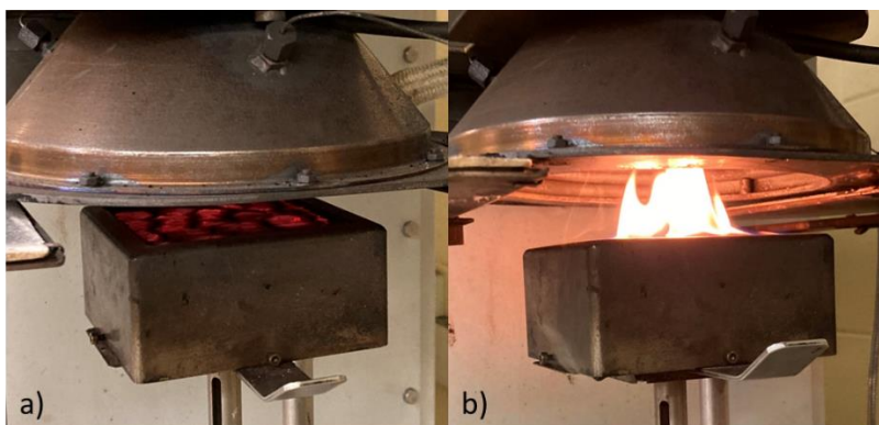
Figure 2.3: a) Smouldering combustion and b) flaming combustion (author's photos)
