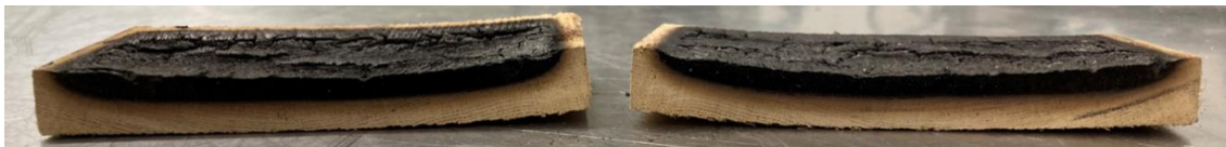
Figure 4.10: Char layer of a wet sample (W20-1) (author's photo)
