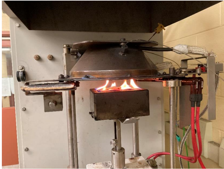
Figure 4.5: Cone calorimeter test in progress (author's photo)
