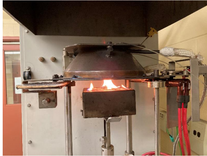
Figure 2.4: Cone calorimeter test in progress (author's photo)
