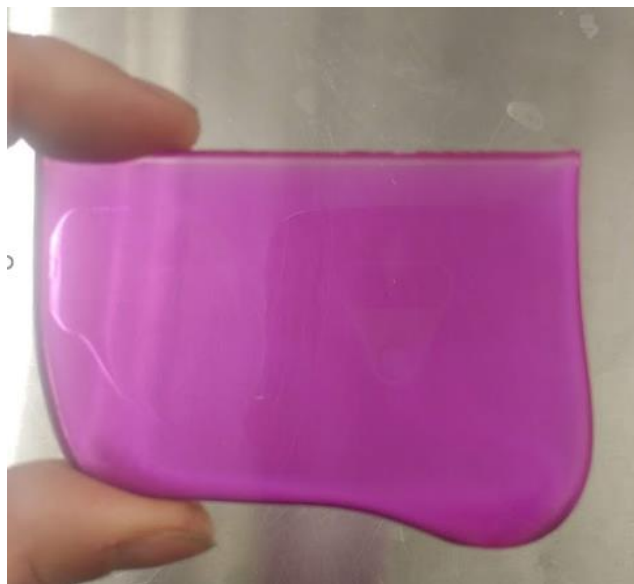
Figure 9.2. Waveguide sample after being removed from the mould
