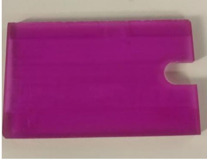
Figure 9.3. Waveguide sample after machining
