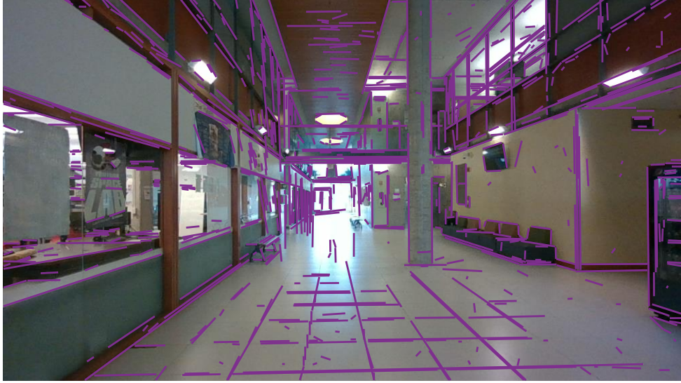
Figure 4.2: Image from York-RGBD-LiDAR dataset overlaid with line segments (purple) detected with MCMLSD algorithm [45].
