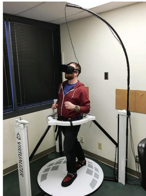
Fig 5.3. from Ekstrom et al., 2018. Example of an omnidirectional setup, with an HMD to control the visual stimuli.
