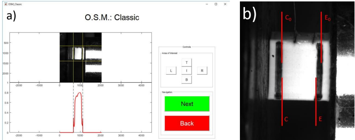
Figure 3-2: Image showing calculation of strain in OSM-Classic software. (a) Image of software with sample showing the Region of Interest; (b) the sample with marks for tracking, C and E represent the current edges, while C_0 and E_0 are the initial positions of the edges.
