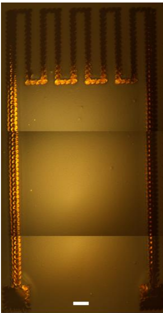
Figure 3-8: Optical micrograph of the revised fabricated strain gauge with wider and longer lines as well as with two parallel lines. The scale bar represent 250\ \mu\text{m} .
