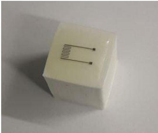
Figure 3-9: The fabricated sample; the strain gauge printed onto the adhesive on one side of the 3D printed 10 mm cube.
