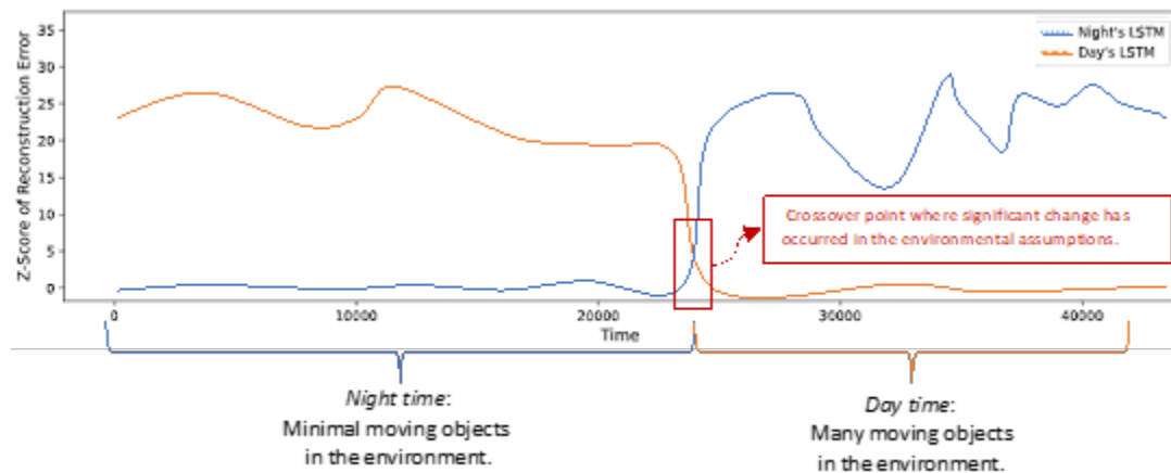
Figure 6.4: Starting at midnight, the Z-Scores of reconstructed RSSI values corresponding to the transmitting node s using the two trained models (for day and night) is tracked. At about dawn, when occupants started to wake up and move about, the error rate of the night model significantly increases while the day model’s error rate drops significantly.
