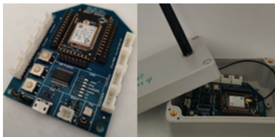
Figure 6.5: Digi XBee 3 Series programmable module implementing IEEE 802.15.4. [86] in a weatherproof secure enclosure protecting the devices from elements when deployed.
