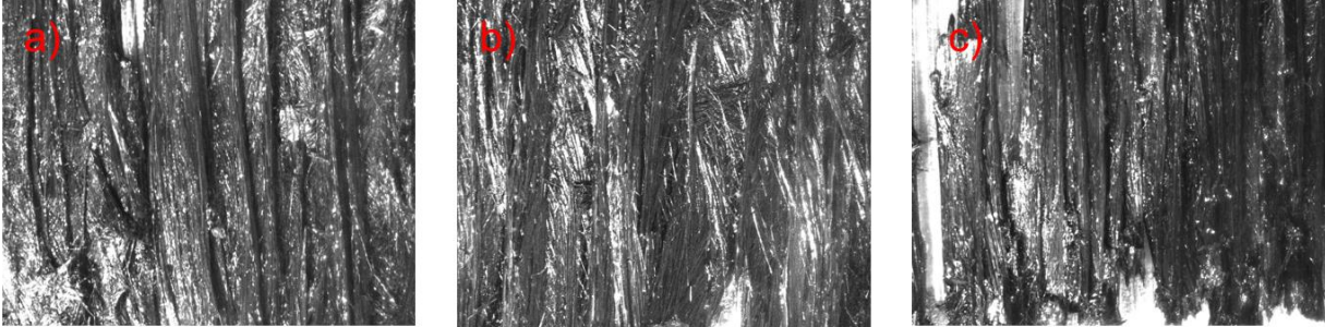
Figure 5-9: Images of a layer of pitch carbon fiber printed at a raster spacing 1 mm, the samples were printed at a) 800 mm/min, b) 1500 mm/min, and c) 3000 mm/min.
