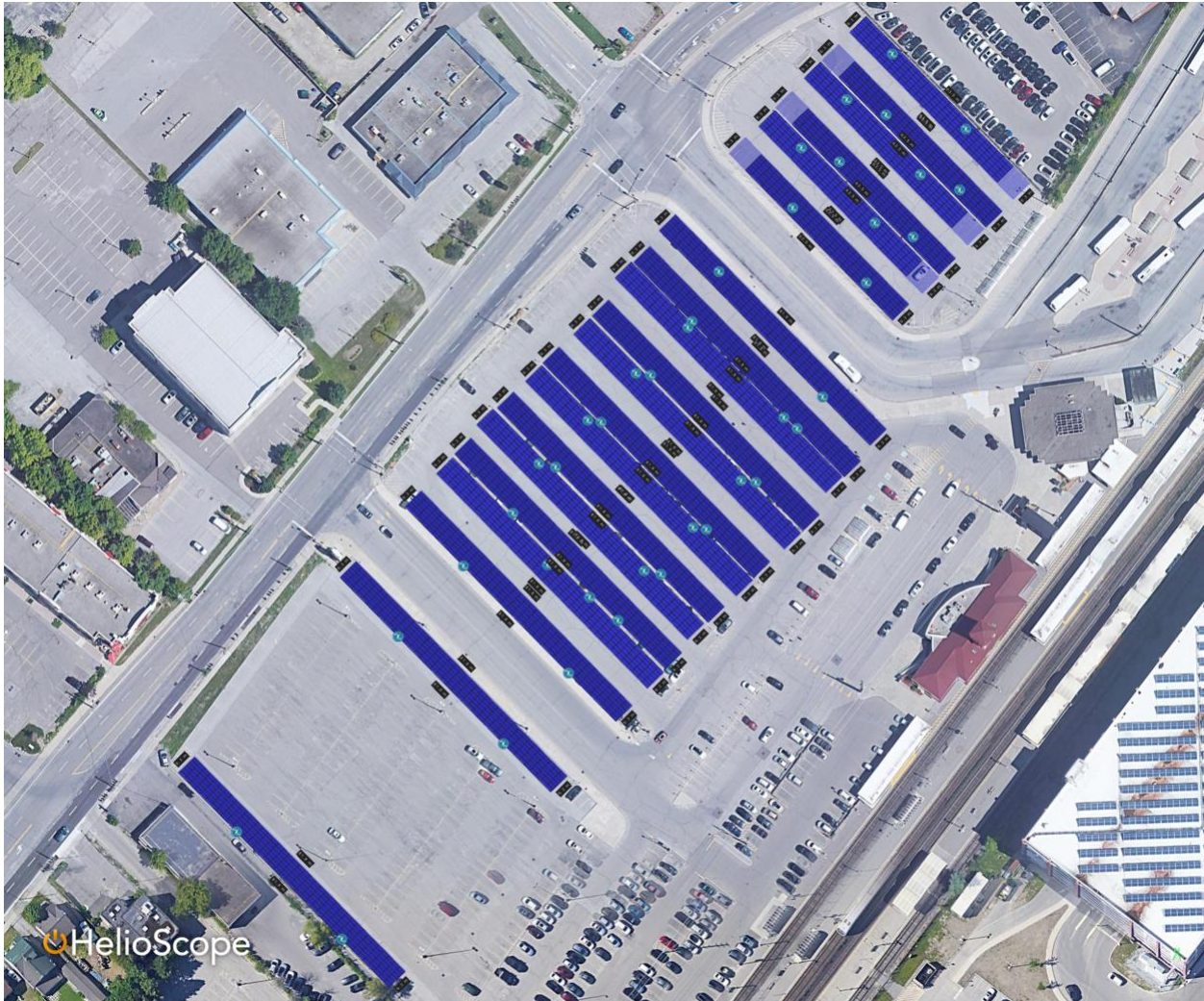
Figure 9. HelioScope Solar PV Model for Oakville GO Station. System Model Image.
